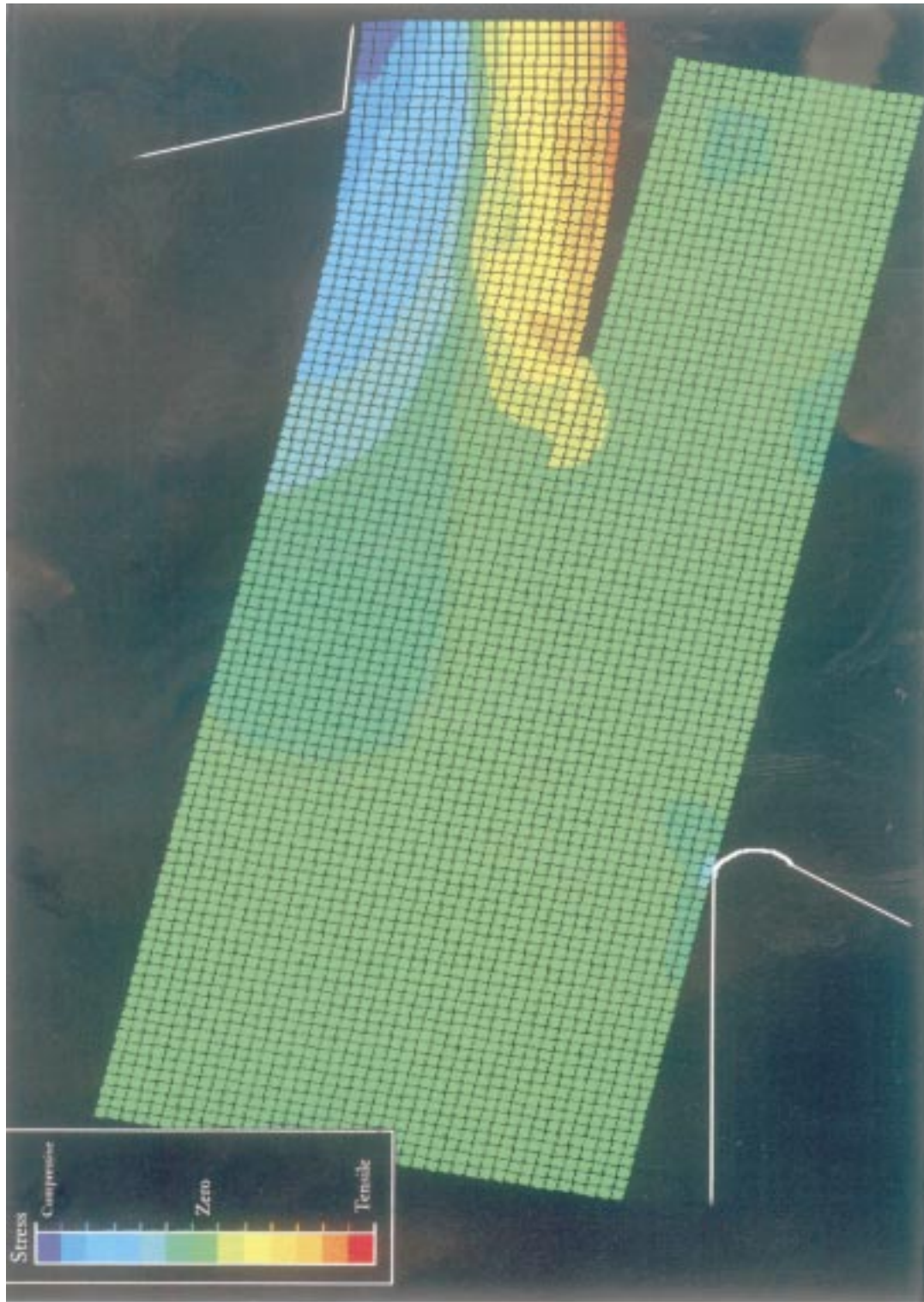
Fig. 4. Graphic representation of crack propagation in the tied model.
